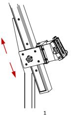
**Step 3** Secure the cameras on the mounts.
