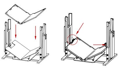
**Step 3** Insert the roof base to the legs and lock it with 4 screws on each side.
