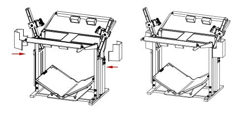
**Step 8** Place shade on the roof base and the lighting panels.
