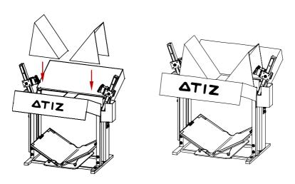
**Step 10** Attach the black plate to the end of the arm. The black plate will block the view of ceiling from appearing in the scene.
