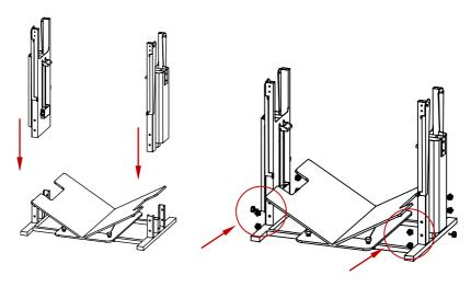
**Step 2** Put the V glass on the cradle and lock the V glass to the connectors with 2 knobs on each side.
