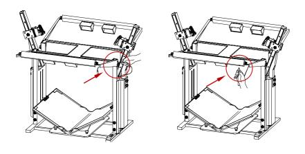
**Step 7** Attach the arm covers to the top part of the legs. The magnets on the covers will hold to the legs.
