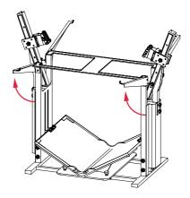
**Step 6** Hang the lighting panels on the hangers and lock them with a knob on each side.
