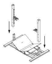
2. Tighten 3 knobs on the front, 3 knobs on the rear and 2 knobs on the inner side of each leg.
