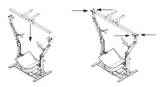
8. Attach the lamps to the lamp hanger. Tighten the knobs on both lamps. Plug the AC cord into each lamp.
