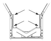
6. Straighten the top bar. Attech the lighting hanger to the top bar and tighten the 2 knobs.
