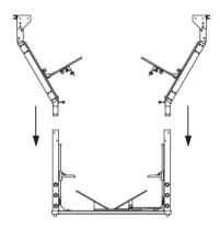
4. Fix the V glass with the arm connector. Tighten 2 knobs with nuts at each left and right side.
