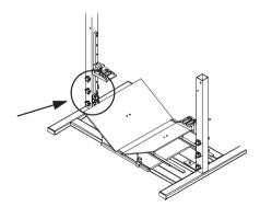
Connect the arm to the leg. The sticker on the end of the arm should match with the sticker on the end of the leg. Then tighten the knobs. Repeat on the other side.
