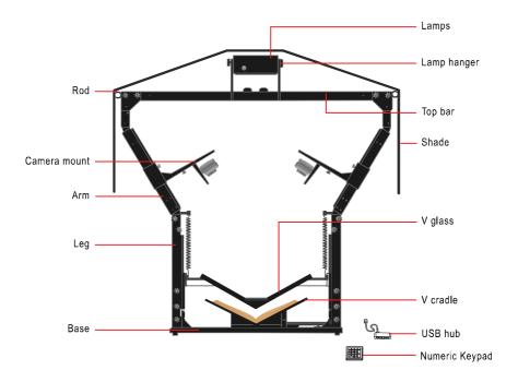
Step 1 Place the base on the table and connect the left and right legs to the base as shown.
