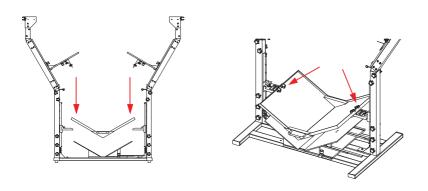
Step 5 Install the springs on both sides.
