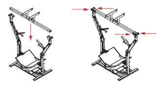
Step 8 Attach the lamps to the lamp hanger. Tighten the knobs on both lamps. Plug the AC cord into each lamp.
