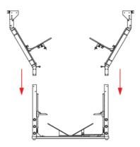
Step 4 Fix the V glass with the arm connector. Tighten 2 knobs with nuts at each left and right side.
