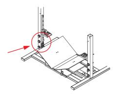
Step 3 Connect the arm to the leg. The sticker on the end of the arm should match with the sticker on the end of the leg. Then tighten the knobs. Repeat on the other side.
