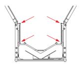
Step 6 Straighten the top bar. Attach the lighting hanger to the top bar and tighten the 2 knobs.
