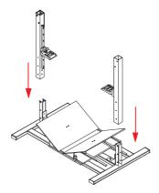
Tighten 3 knobs on the front, 3 knobs on the rear and 2 knobs on the inner Step 2 side of each leg.
