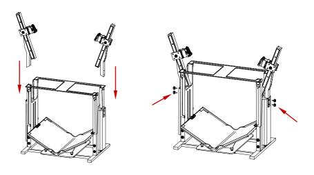
**Step 5** Move light hangers in the front and the rear upward to their positions and lock them with knobs.
