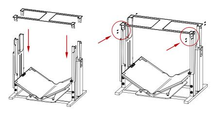
**Step 4** Connect the arms to the legs and lock the arms with 2 knobs on each arm.
