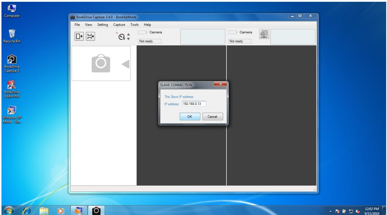
9. Now it's time to connect the cameras. Make sure both cameras remain off while the USB cables are plugged to the appropriate PC port. (Right camera connected to the Master PC and Left camera connected to the Slave PC). First turn on the right camera. Wait until it is connected to the Master PC on BookDrive Capture. Then, turn on the left camera.
