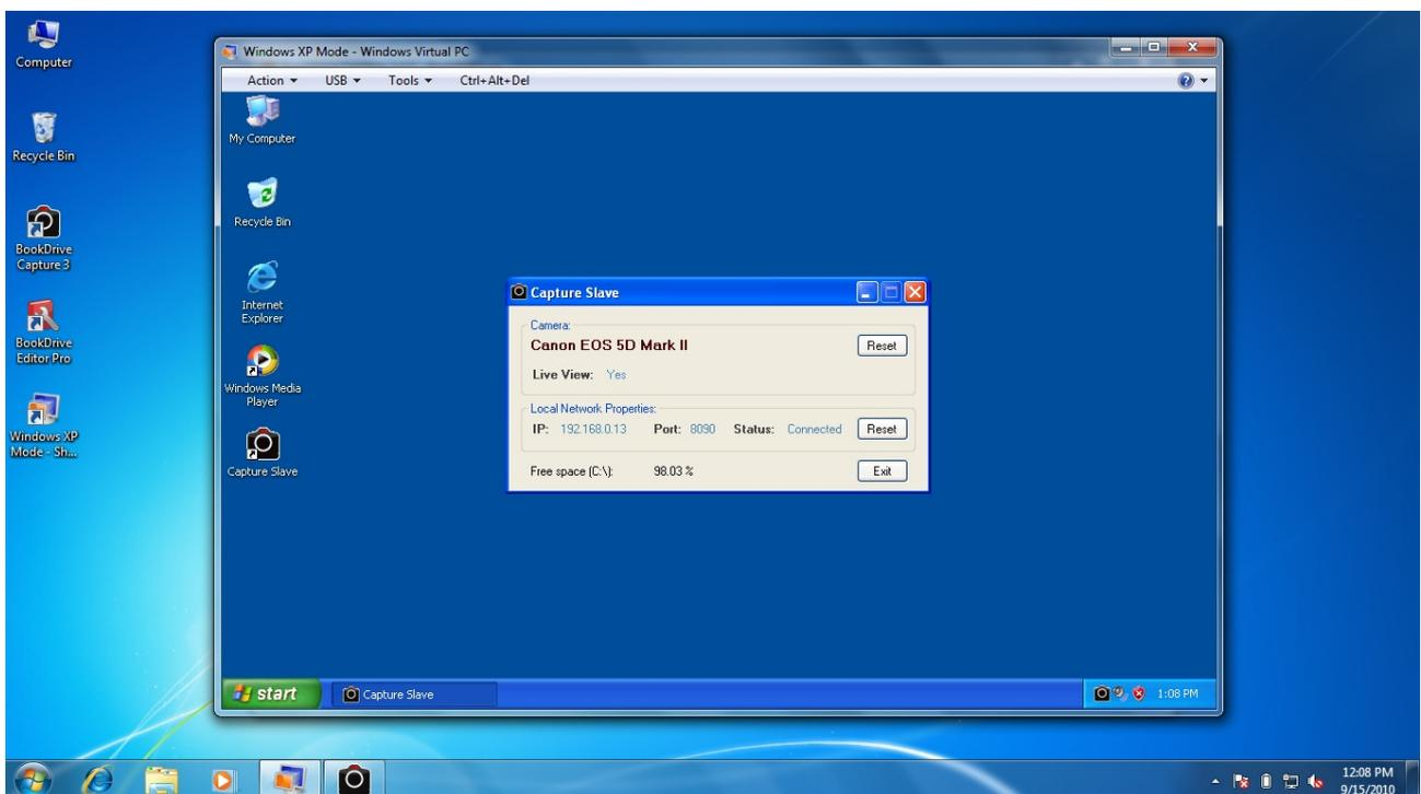
You can do quick testing of the connection by Right Click on the Capture Slave program and select **Capture**. If the camera is properly connected, the program will order the left camera to shoot.
