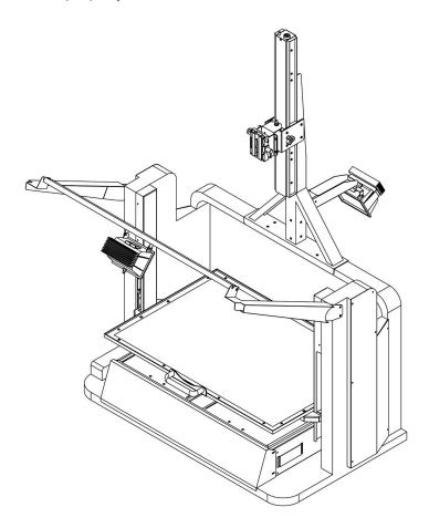
5. Attach the body shade to the machine as shown below.
