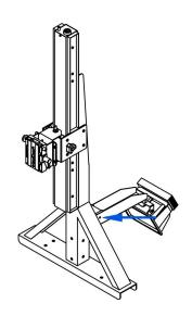
3.2 Connect the main camera mounting arm to its slot located at the top back part of the machine.
