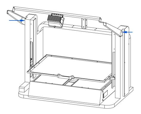
2.2 connect the LED light bar on the light hangers and lock it with knobs.
