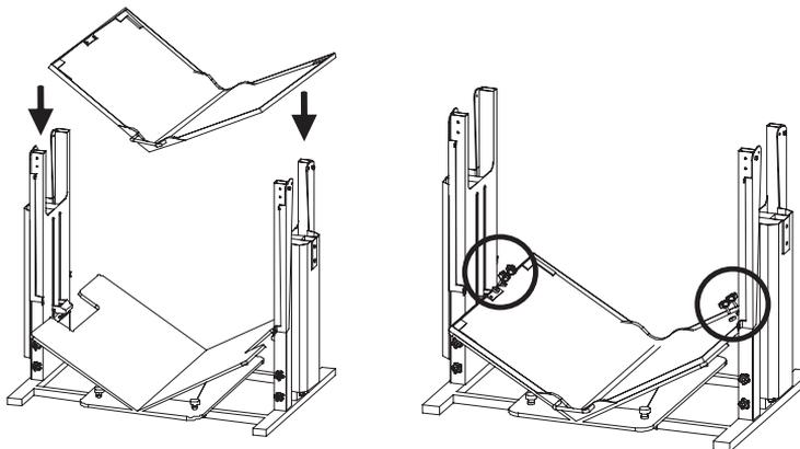
3. Insert the roof base to the legs and lock it with 4 screws on each side.
