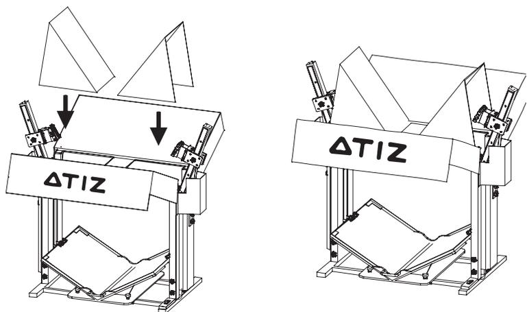
10. Attach the black plate to the end of the arm. The black plate will block the view of ceiling from appearing in the scene.
