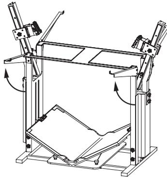
6. Hang the lighting panels on the hangers and lock them with a knob on each side.
