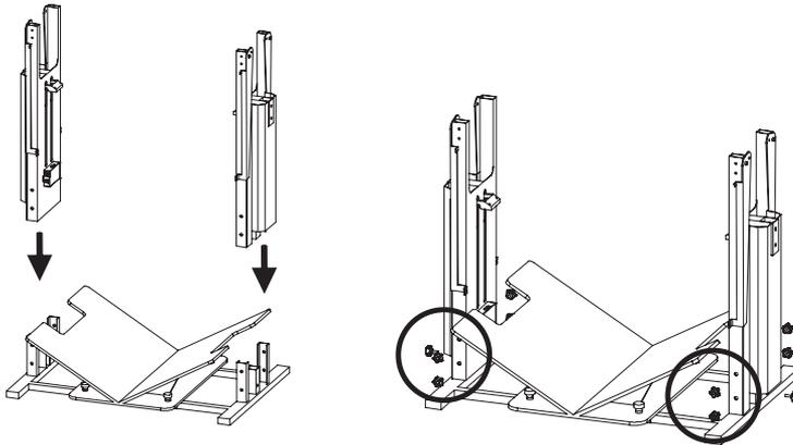
2. Put the V glass on the cradle and lock the V glass to the connectors with 2 knobs on each side
