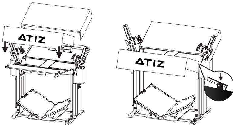
9. Put the roof on the roof base like this.
