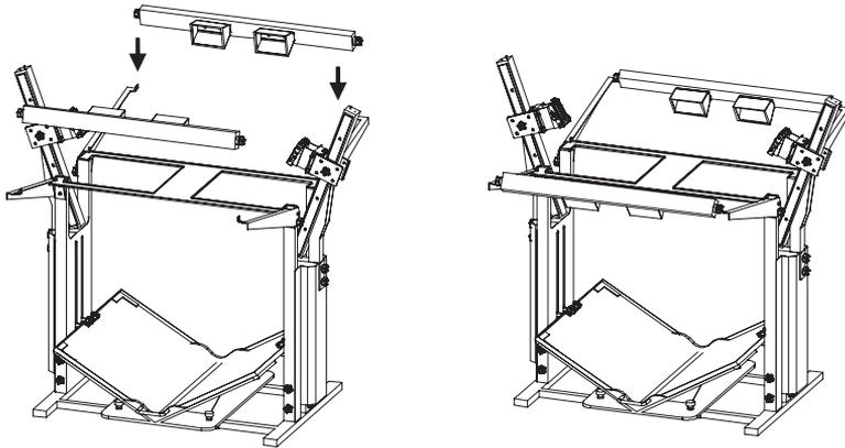
7. Attach the arm cover to the top part of the legs. The magnets on the covers will hold to the legs.
