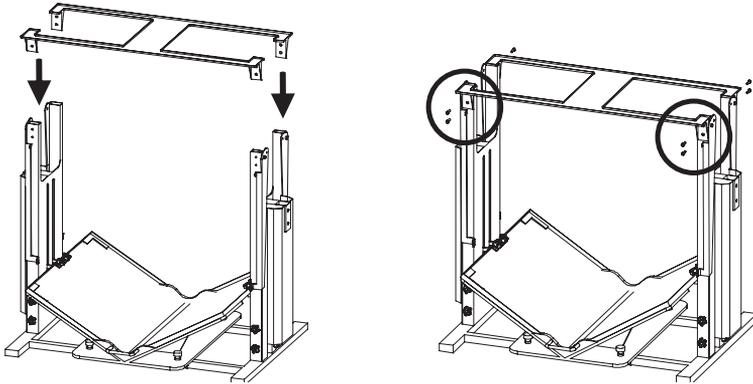
4. Connect the arms to the legs and lock the arms with 2 knobs on each arm.
