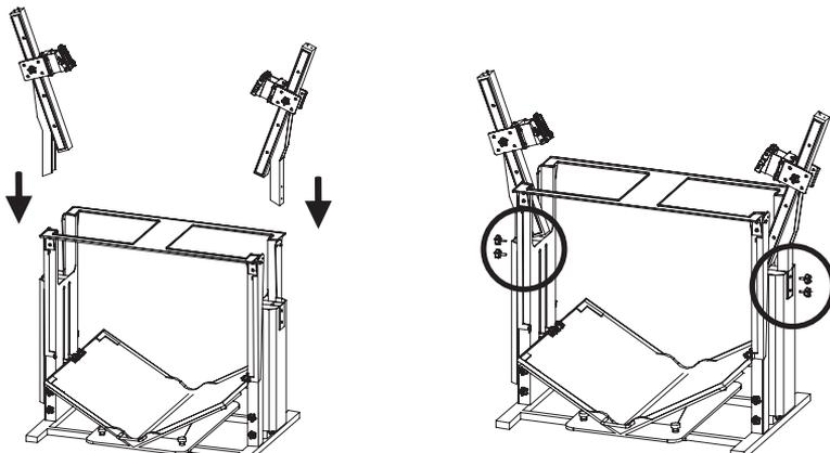
5. Move light hangers in the front and the rear upward to their positions and lock them with knobs.
