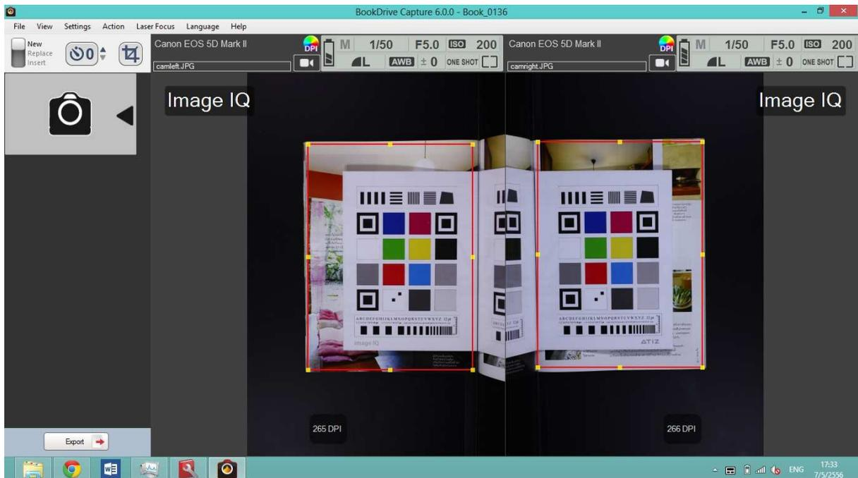
6. If program cannot calibrate, program represents text "Not found Image IQ". Please adjust and center image IQ in order to be functional perfectly. The procedure will be repeated until the software display the correct number of DPI.
